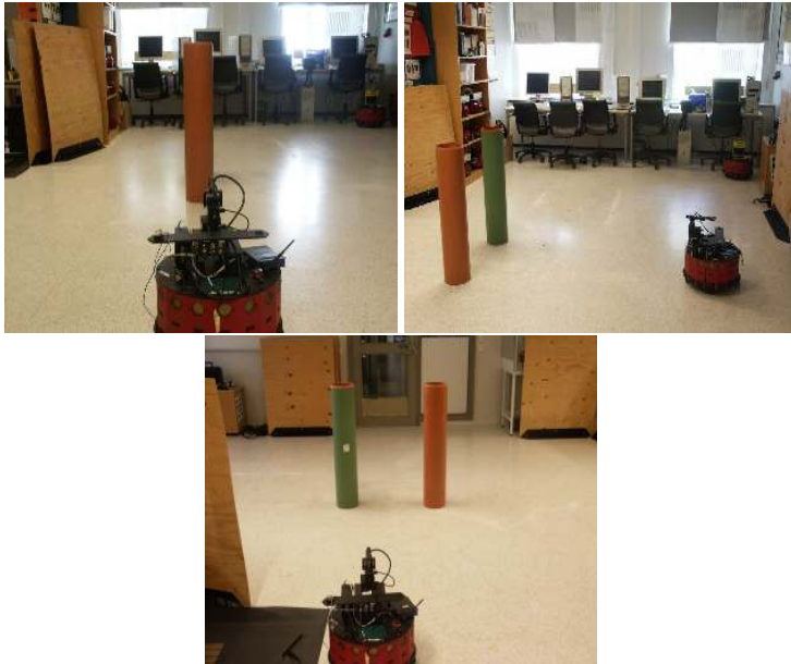
Figure 7.2: Trying to identify a marked gas bottle. Left: From her initial position, Pippi perceives only one candidate object \pi_1 but without a mark. Right: Pippi perceives a second candidate \pi_2 , while trying to observe a mark on the first one from another observation position. Bottom image: Pippi observes a mark on the second candidate \pi_2 , which results in anchoring the requested object to \pi_2
