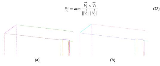
Figure 11. Comparison of 3D line segments before and after merging. (a) Before merging. (b) After merging.
