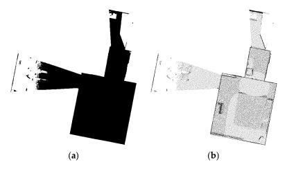
**Figure 3.** Comparison of the original point cloud and the subsampled point cloud projected to the X-Y plane. (a) Projection of the original point cloud. (b) Projection of point cloud after subsampling.
