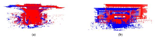
Figure 23. The registered point cloud on the X-Y plane. (a) Top view. (b) Front view.
