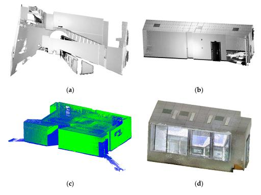
Figure 12. Raw point cloud data. (a) Staircase. (b) Corridor. (c) Laboratory. (d) Lounge.
