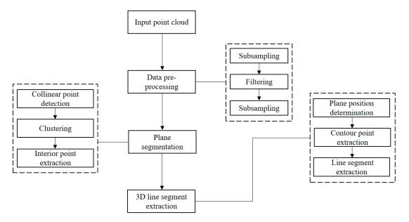
Figure 1. Overall flow of the proposed 3D line segment feature extraction method.
