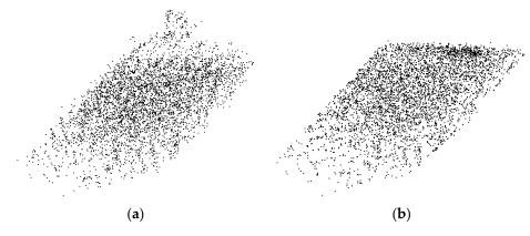
**Figure 9.** Comparison of the original planar point cloud and the projected point cloud. (**a**) The original planar point cloud. (**b**) The projected planar point cloud.
