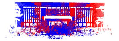
**Figure 24.** The final registration results. Red part is the target point cloud, and blue part is the point cloud to be matched.
