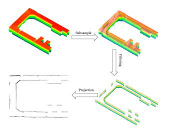
**Figure 2.** A demonstration of the raw data pre-processing flow. Point cloud is colored in the Z-axis direction.
