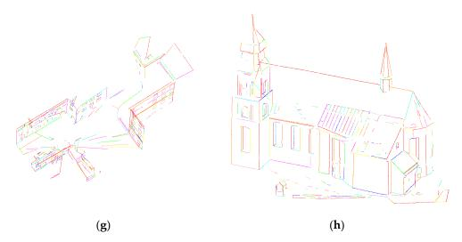
**Figure 16.** Effects of two outdoor scenes on plane segmentation, contour point extraction and 3D line segment extraction. The first column corresponds to Birdfountain and the second column corresponds to Bildstein. (**a**,**b**) are the input outdoor scenes. (**c**,**d**) are the plane segmentation results. (**e**,**f**) are the extracted contour points. (**g**,**h**) are the extracted 3D line segments.
