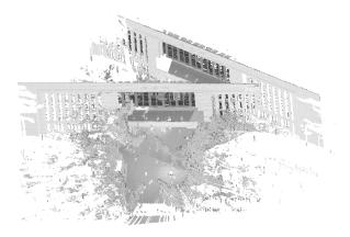
**Figure 19.** The target point cloud and the point cloud to be registered; the front is the point cloud to be registered, and the back is the target point cloud.
