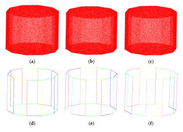
**Figure 17.** Three-dimensional line extraction effect under gaussian noise interference, from left to right are 0.01 m, 0.03 m, and 0.05 m Gaussian noise, respectively. (**a**,**b**,**c**) Input point clouds with Gaussian noise. (**d**,**e**,**f**) Extracted line segments.
