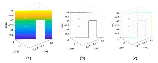
**Figure 10.** A demonstration of extracting 3D line segment from planar point cloud. (**a**) Planar point cloud. (**b**) Extracted contour points. (**c**) Extracted 3D line segments.
