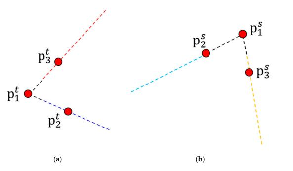
**Figure 18.** Point cloud registration diagram based on 2D line segment. (**a**) Target point cloud segment. (**b**) Point cloud line segments to be registered.
