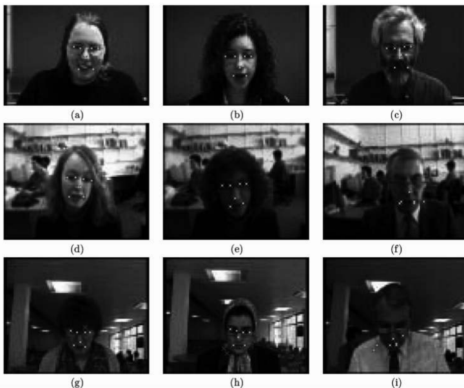
FIG 10. – Samples from sessions 1, 5, and 10 of the English part of the BANCA dataset. The crosses are initial detections, the dots are final landmarks after structural correction. Facial hair as in sample (c) and eyeglasses as in samples (f) and (i) make detection difficult.
