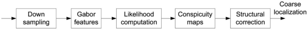
FIG 1. – Coarse landmark localization starts with computation of Gabor wavelets on downsampled images. Conspicuity maps for each landmark are computed by summing the likelihoods under mixtures of factor analyzers models. The most conspicuous locations are sent to the structural analysis subsystem for correction.
