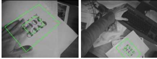
Figure 6. Targets lacking in texture can be localised successfully over a large viewpoint range and in the presence of background clutter and partial occlusion.
