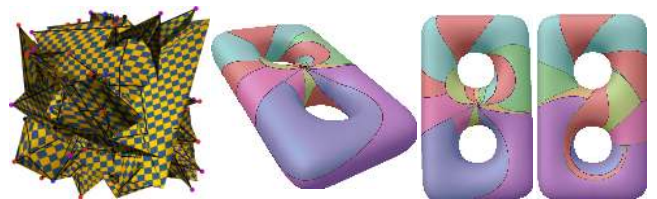
Figure 23: Left: A random mesh sampled from a sphere. Right: Partition for a torus with a single singularity.
