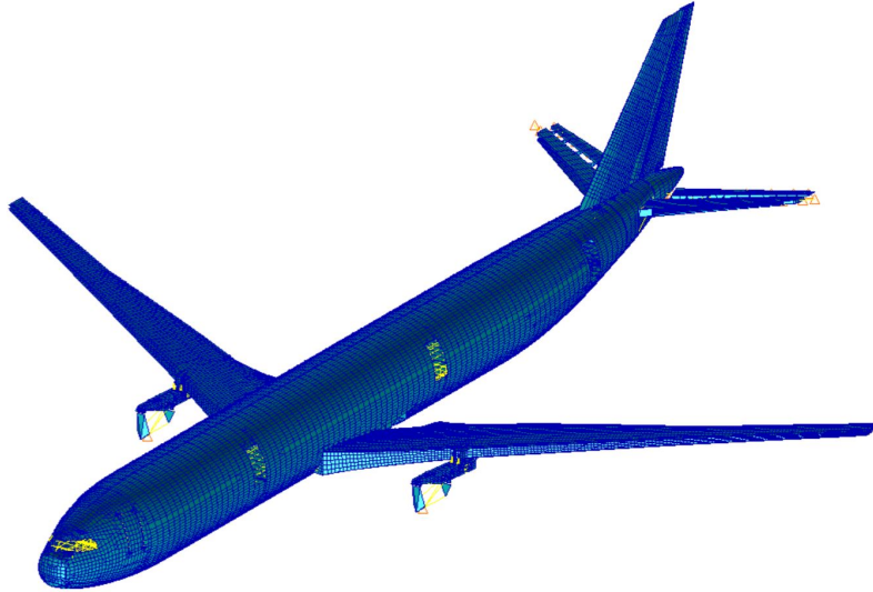
Fig. 1 Finite element model of the XRF1 aircraft concept
