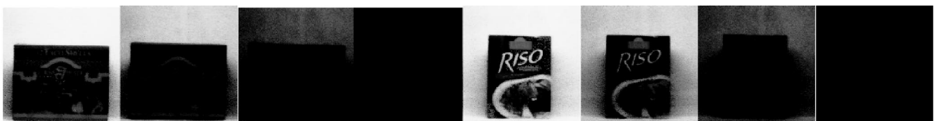
Fig. 6. Two objects under varying illumination intensity generating each four images with SNR \in \{24, 12, 6, 3\} .
