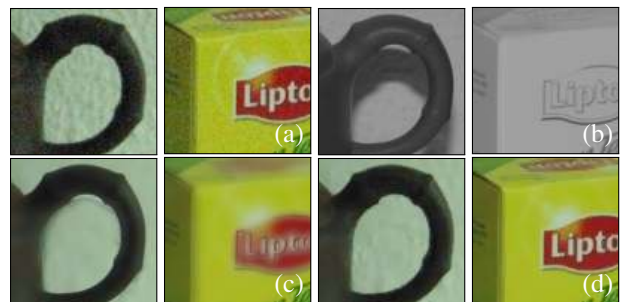
Figure 10. RGB and flash NIR image restoration. (a) RGB images, (b) NIR images, (c) GF [10] [ r = 3 , \varepsilon = 4^{-4} ], (d) ours [ \mathbf{u}^0 = \mathbf{1} , \lambda = 15 , \mu = 60 , \nu = 30 , k = 5 ].
