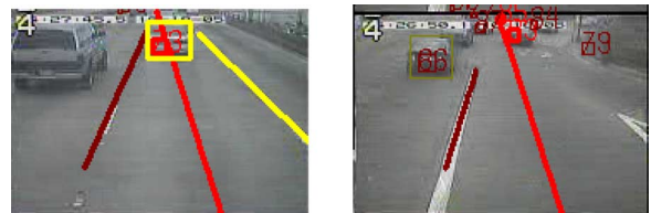
Fig. 16. Preliminary sensor-fusion result of vision-based lane-and-obstacle-detection results, LIDAR, and vehicle navigation information. The obstacles' relative positions with respect to the lane are estimated. The thick red line is a projected vehicle path.
