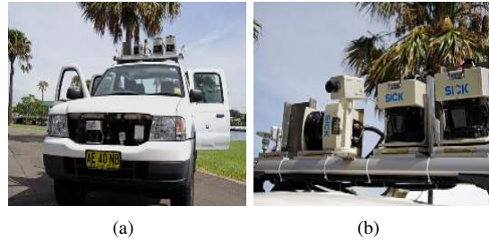
Fig. 1. a) The testbed vehicle and b) the sensors mounted on the roof.
