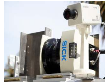
Fig. 8. The camera and vertically mounted laser.
