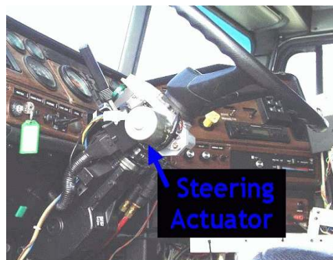
Figure 16: Steering Actuator Mounted on the Steering Column
