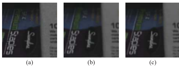
Fig. 6 Images from (a) to (c) are ground truth, output images from the model without OSS module, and with the OSS module.
