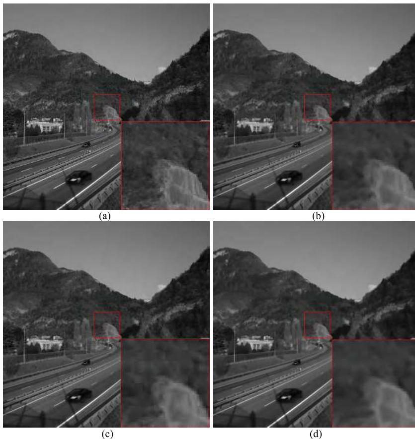
FIGURE 2. The influence on an original image caused by median filtering, JPEG compression, and image deblocking. (a) an original image; (b) its 3 \times 3 median filtered image; (c) a compressed image generated by performing JPEG compression on the filtered image with a quality factor (QF) of 70; (d) this compressed image were performed image deblocking.
