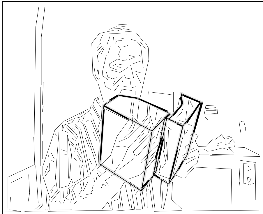
Figure 6: The model is shown following the third and final iteration of parameter determination. The region of uncertainty around each model edge is now very small.
