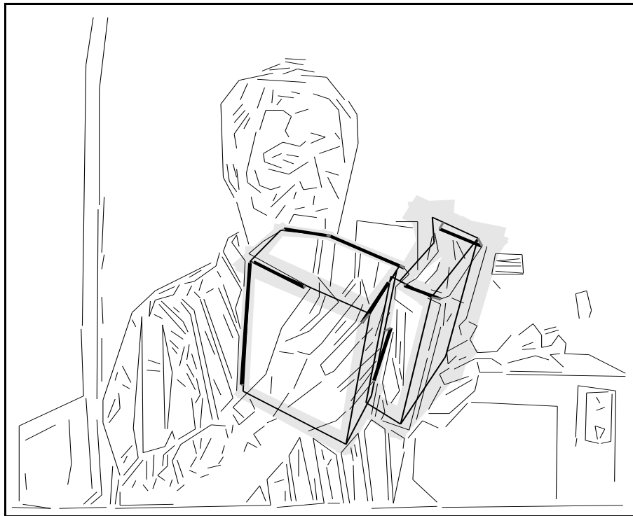
Figure 4: The position of the model is shown following the first iteration of matching and parameter determination. Further matched image segments are shown with heavy lines.
