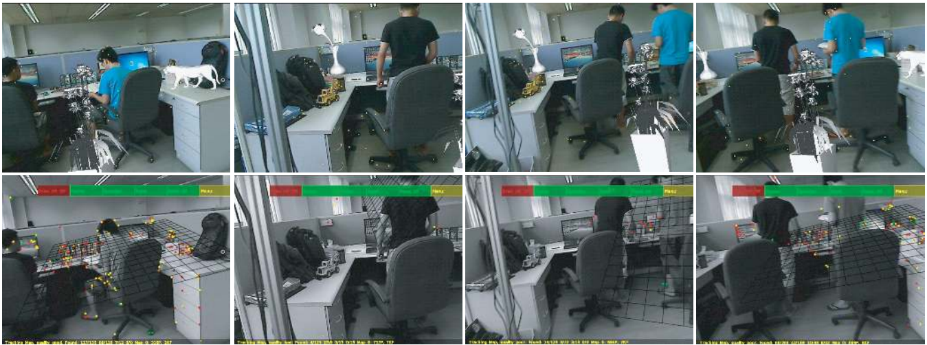
Figure 11: “Two-Men” example. Top: the SLAM result (with augmented reality) of our system. Bottom: the SLAM result of PTAM.
