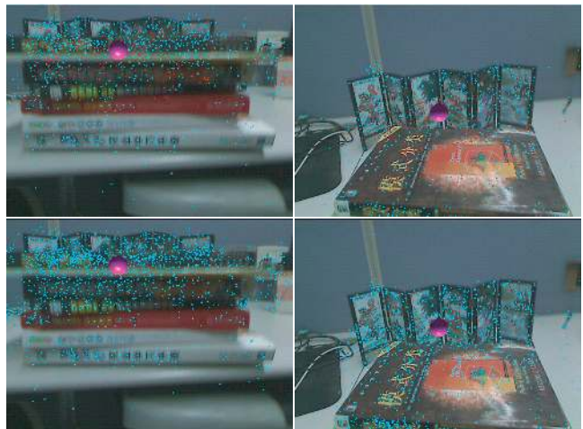
Figure 5: Handling occlusions caused by static objects. Top: the SLAM result without occlusion handling. The valid 3D points are highlighted with cyan color. Many 3D points are recognized as “invalid” 3D points (highlighted with red color) due to occlusions. Bottom: the SLAM result with occlusion handling. Most of the occluded points are successfully identified and not set to invalid.
