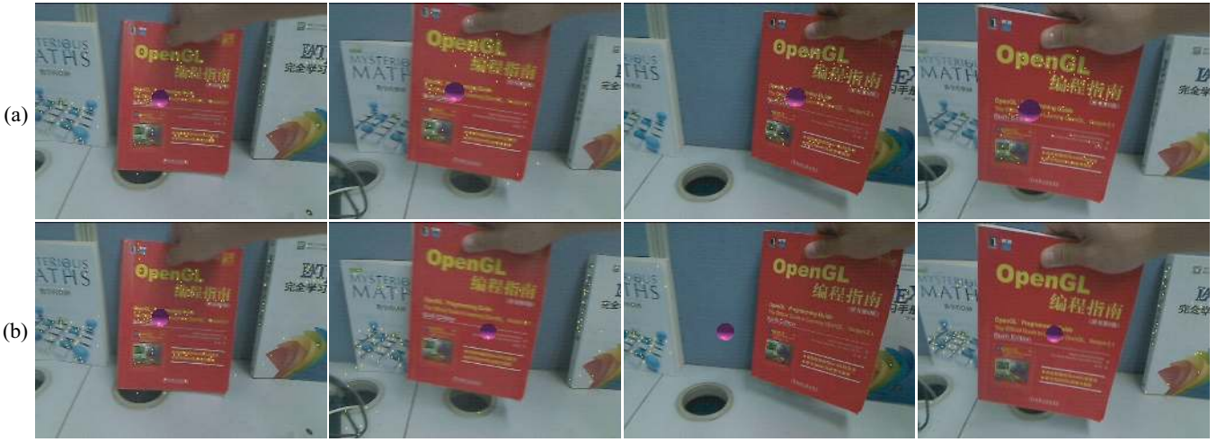
Figure 8: SLAM result comparison with different robust estimators. (a) The SLAM result with standard RANSAC. The inserted purple sphere drifts with the moving red book, which is not accurate. (b) The SLAM result with our PARSAC. The inserted purple sphere stays at accurate position without drift.
