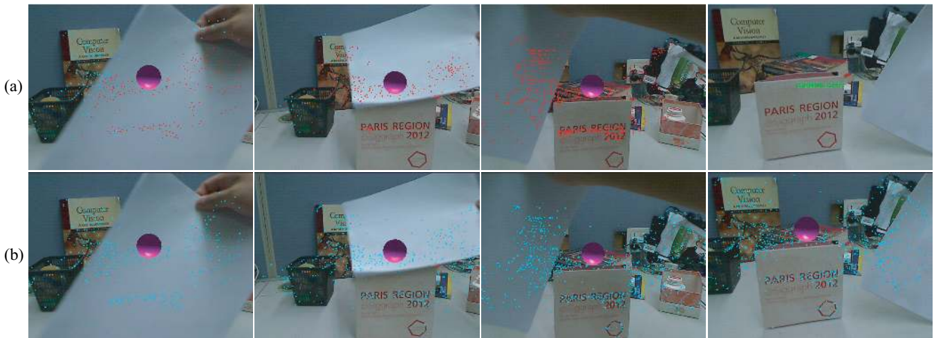
Figure 4: Handling occlusions caused by dynamic objects. (a) The SLAM result without occlusion handling. The valid 3D points are highlighted with cyan color. Since most 3D points are recognized as “invalid” 3D points (highlighted with red color) due to occlusions caused by a moving paper, the estimated camera may frequently drift or even lost. (b) The SLAM result with occlusion handling. Almost all the occluded points are successfully identified and not set to invalid, so the camera poses can be reliably estimated.
