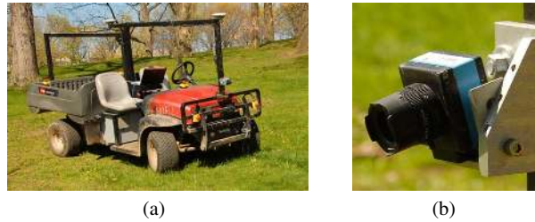
Fig. 4 (a) Our robot, and (b) A monocular camera attached in front of the robot.
