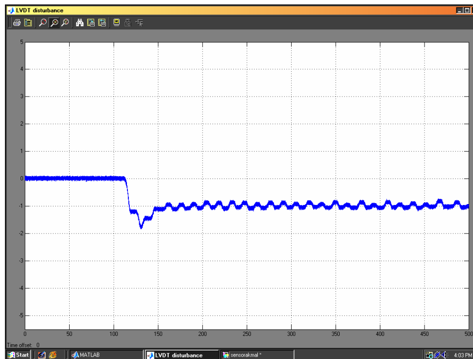
PID scheme ( P=7 I=13 D=48 ) with changed set value from 0 to -1
