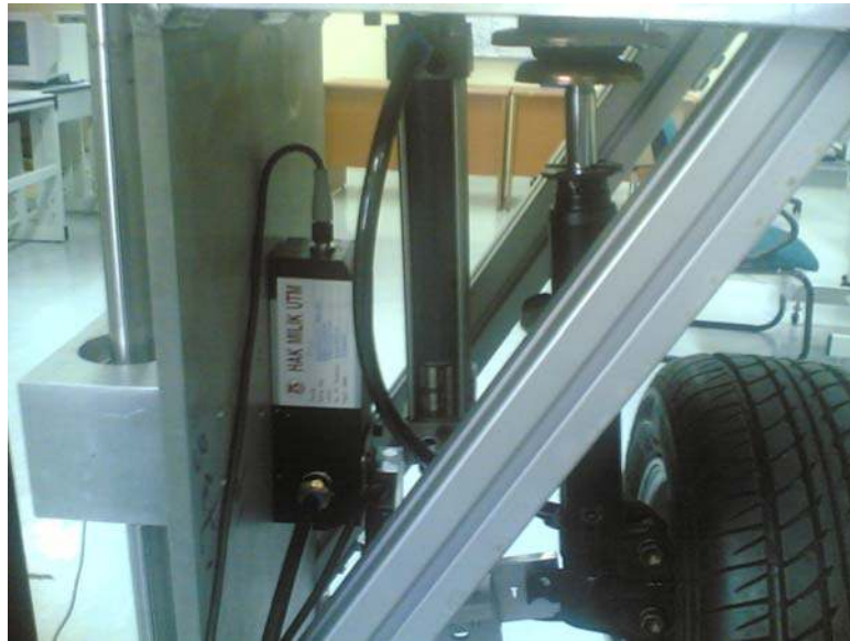
Sensors installation (laser sensor and LVDT)
