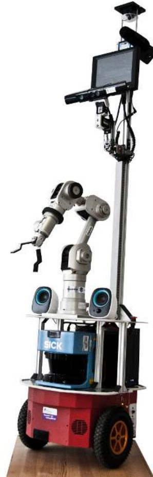
Fig. 1 – Kate , the service robot providing the platform for the application of the proposed method.
