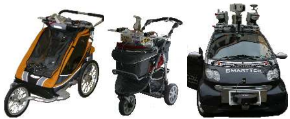
Fig. 1. Mobile recording platforms used in our experiments. Note that in this paper we only employ image information from a stereo camera pair and do not make use of other sensors such as GPS or LIDAR.
