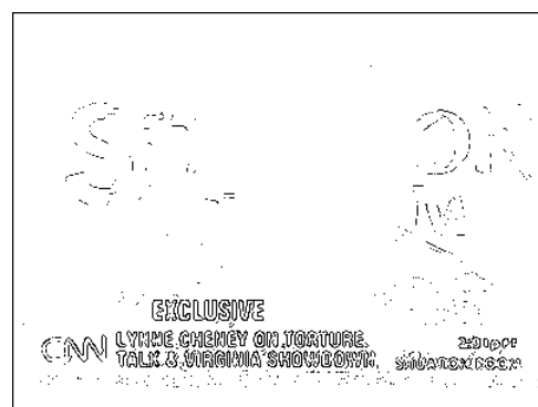
Fig. 5. The AND-edge-map: the result after taking AND operation on four Canny edge maps of Fig. 4.
