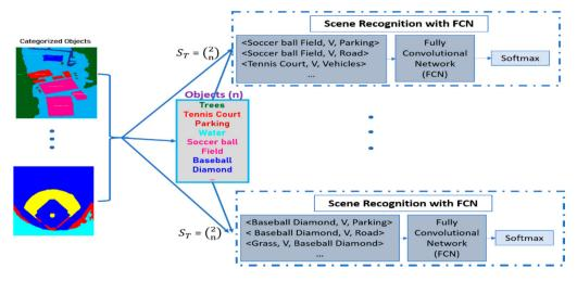
Figure 8. Schematic view of OORs between object triplets present in the remote sensing imagery.
