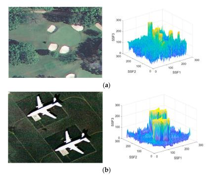
**Figure 5.** Spectral–spatial feature representation: (**a**) original image (left) and corresponding SSF extraction (right) from UCM dataset; (**b**) original image (left) and corresponding SSF extraction (right) from AID.
