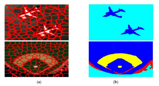
**Figure 6.** Results of super-pixel patterns on some remote sensing images from UCM dataset: (**a**) super-pixels patterns applied on UCM images; (**b**) homogeneous regions extracted from super-pixel patterns.
