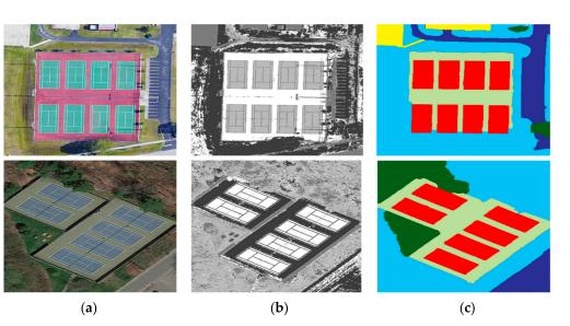
**Figure 3.** MRF labeling of segmented images over AID: (**a**) original image; (**b**) segmented image; (**c**) labeled via MRF.
