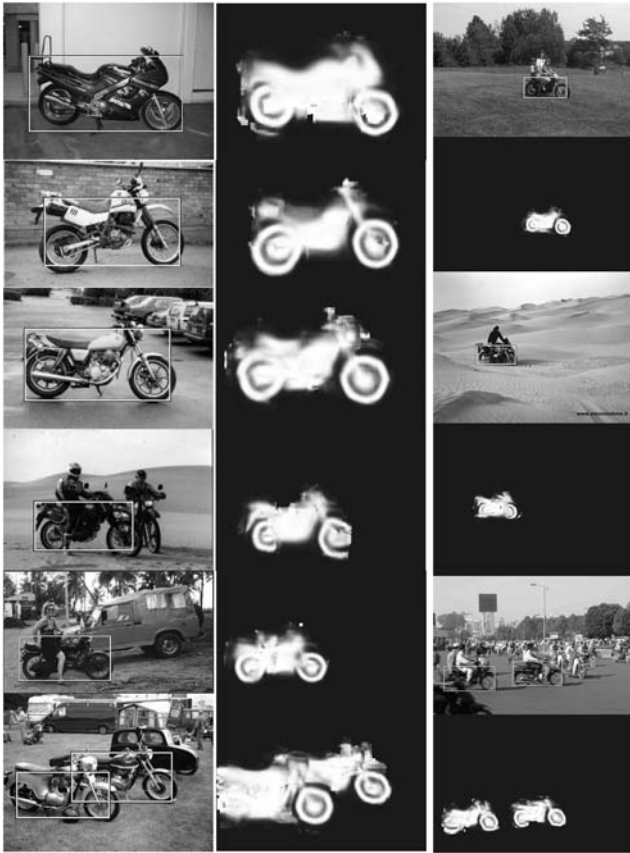
Fig. 18 Examples for the variety of motorbike shapes and appearances that are still reliably detected and segmented
