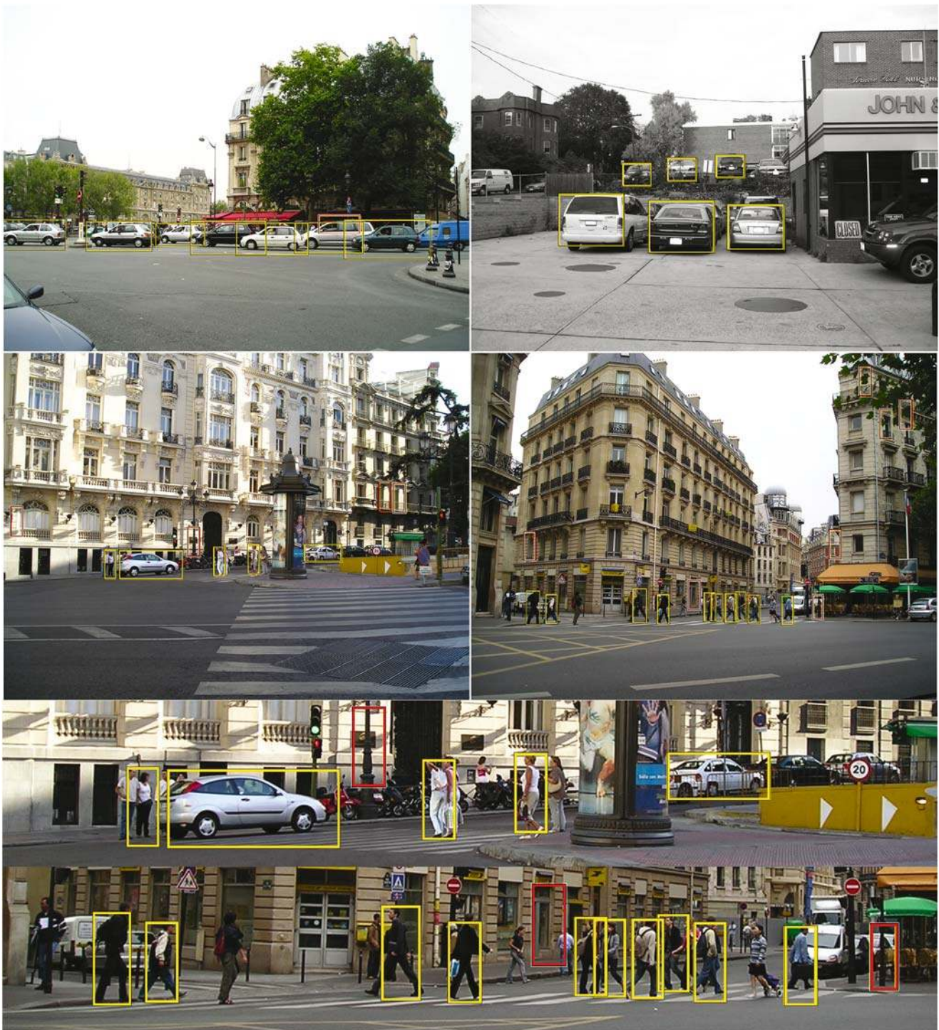
Fig. 23 Example detections on difficult test images from the MIT LabelMe data set (Russell et al. 2005). All images were processed at their original resolution of 2048 \times 1536 pixels. The results confirm our ap-
