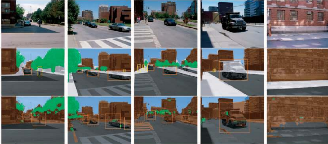
Fig. 10. Top row: Sample StreetScenes examples. Middle row: True hand-labeling; color overlay indicates texture-based objects and bounding rectangles indicate shape-based objects. Note that pixels may have multiple labels due to overlapping objects or no label at all (indicated in white). Bottom row: Results obtained with a system trained on examples like (but not including) those in the second row.
