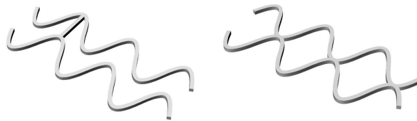
Figure 3: Copy and mirror stent designs
