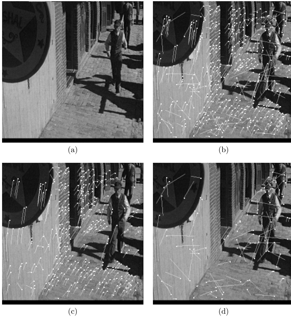
Fig. 7 Fundamental matrix and motion estimation from an image sequence of a camera panning to follow a moving person: (a) shows one of these images, (b) shows the motion vectors obtained from correspondences superimposed on this image, (c) shows correspondences consistent with the estimated epipolar geometry (represented by the fundamental matrix), and (d) shows correspondences inconsistent with the estimated epipolar geometry. Reprinted from International Journal of Computer Vision 24, P. Torr and D. Murray, The Development and Comparison of Robust Methods for Estimating the Fundamental Matrix, 1997, pp. 271–300, with permission from Kluwer Academic Publishers.
