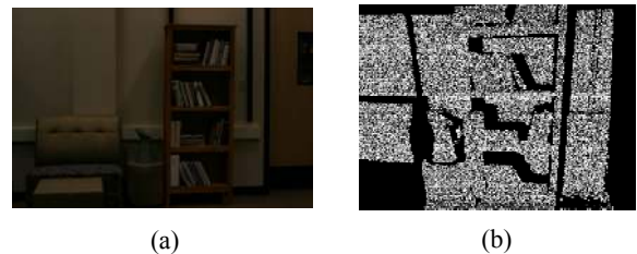
Figure 12. Ambient Lighting. For a scene under significant ambient lighting, our method still performs well: a) a picture of the scene taken under ambient light and b) a reconstructed point cloud using our method.
