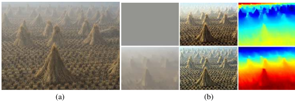
Figure 4: Performance of pixel-wise A . (a) Input image. (b) 1 st row: ATM [29] using global A , 2 nd row: proposed method using pixel-wise A , 1 st column: atmospheric light, 2 nd column: dehazing results, 3 rd column: transmission.
