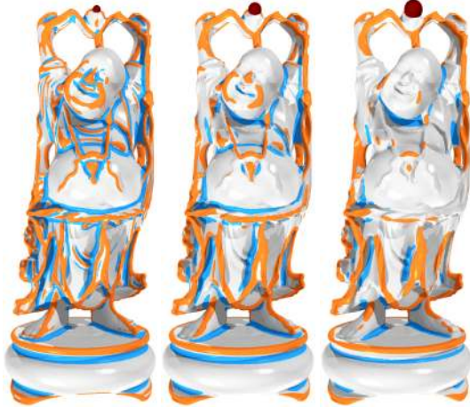
Figure 8: Feature extraction using principal curvatures obtained with PCA on the sphere neighborhood.
