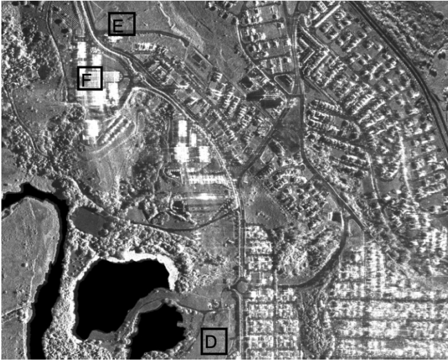
Fig. 4. OrbiSAR image used in the regression models showing the tested regions. Regions D, E, and F represent an open area, a road, and an urban land type, respectively.
