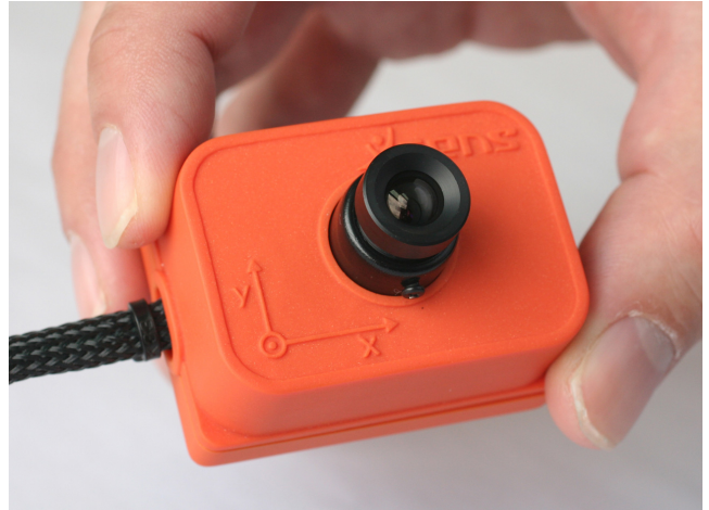
Fig. 1 A prototype of the MATRIS project, integrating a camera and an IMU in a single housing. It provides a hardware synchronized stream of video and inertial data.
