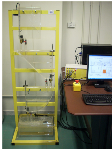
Fig. 8. The laboratory-size three-tank system.
