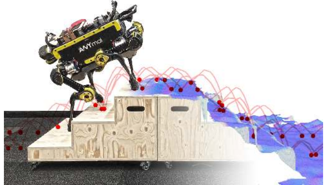
Fig. 1. The robot ANYmal [4] climbing a set of standardized stairs (17 cm \times 29 cm). With help of onboard sensors, a terrain map is generated to plan the footholds (red dots) and base and leg motions (red lines). A video is available at https://youtu.be/CpzQu25iLa0 .
