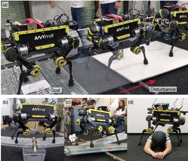
Fig. 11. (a) The robot replans the motion to adapt to the disturbance which has been introduced by relocating the board during execution. In this demonstration, the robot localizes itself with the rotating laser range sensor and can robustly track and reach the desired goal location. (b)–(d) Various experiments demonstrating the versatility and robustness of our approach.
