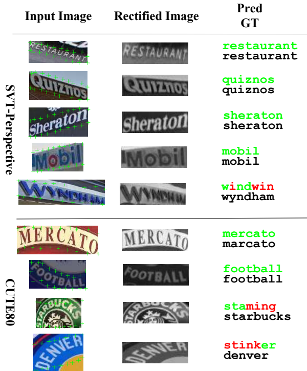
Figure 9. Examples showing the rectifications our model makes and the recognition results. The left column is the input images, where green crosses are the predicted fiducial points. The middle column is the rectified images (we use gray-scale images for recognition). The right column is the recognized text and the ground truth text. Green and red characters are correctly and mistakenly recognized characters, respectively. The first five rows are taken from SVT-Perspective [29], the rest rows are taken from CUTE80 [30].
