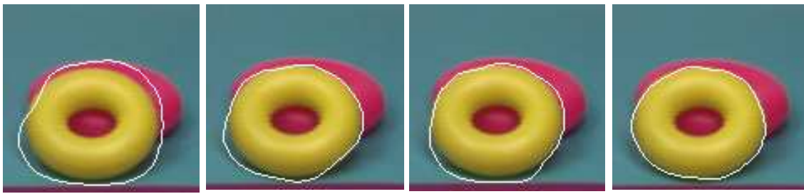
Fig. 3. From left to right a. Colour image with the initial contour as specified by the user (the white contour). b. Segmentation result based on intensity gradient field \nabla I . c. Segmentation result based on RGB gradient field \nabla C_{RGB} . d. Segmentation result based on \theta_1\theta_2 gradient field \nabla C_{\theta_1\theta_2} .
