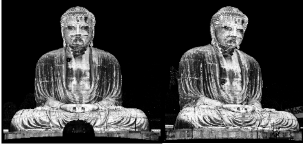
Figure 2. Images using laser reflectance strength as pixel values.
