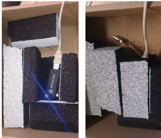
FIGURE 8: The Realtek RTL2832U device was closed inside a box covered by RF absorbers and with the antenna port closed by a 50 Ohm terminator.
