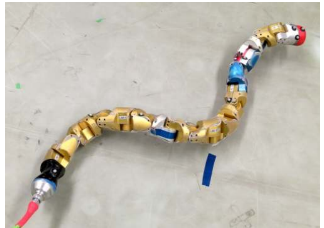
Figure 1: The most recent iteration of the Carnegie Mellon modular snake robot, the Unified Snake . Typically, the robot consists of 16 single degree-of-freedom modules (shown here), with additional unactuated modules at the head and tail.
