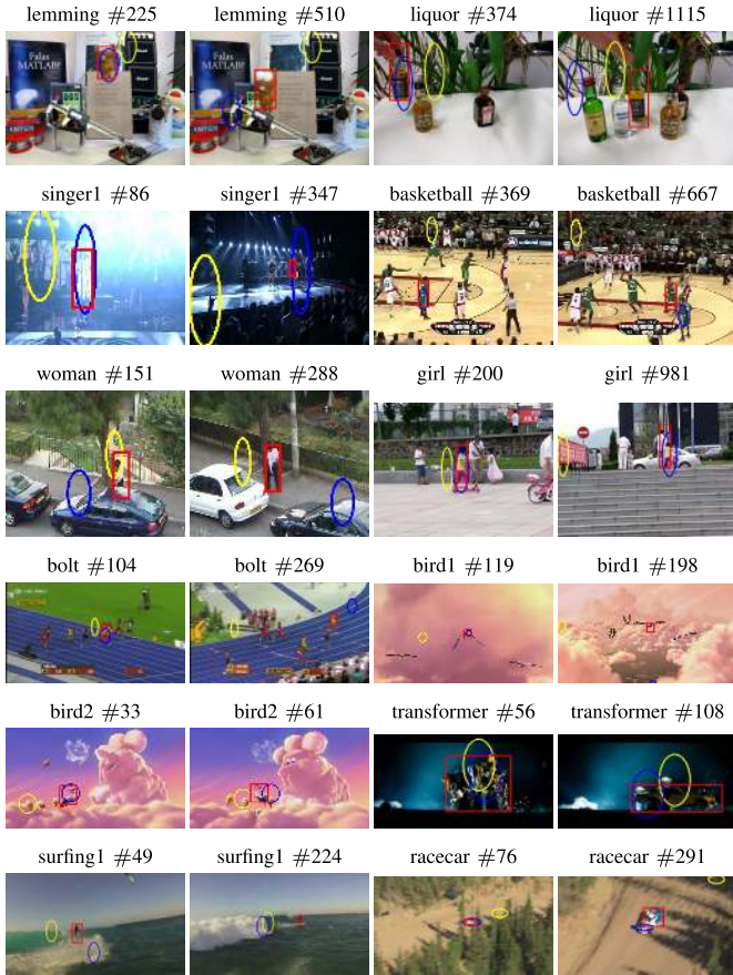
Fig. 7. Tracking results with comparisons to color-based trackers. The results by the MS tracker, the PF method and our algorithm are represented by yellow ellipse, blue ellipse and red rectangles. The proposed tracker is able to handle cluttered background ( girl and basketball ), pose change ( liquor , bolt , bird2 and surfing1 ), scale change ( singer1 and racecar ), heavy occlusion ( lemming , liquor , woman , bird1 , surfing1 and racecar ), shape deformation ( transformer ) and lighting condition change ( singer1 ).
