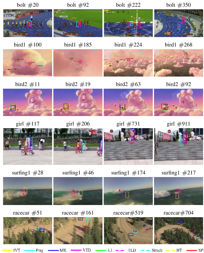
Fig. 9. Tracking results on our own datasets by the IVT, Frag, MIL, VTD, \ell_1 , TLD, Struck, HT and SPT methods. The best four trackers in terms of errors of center location are shown.
