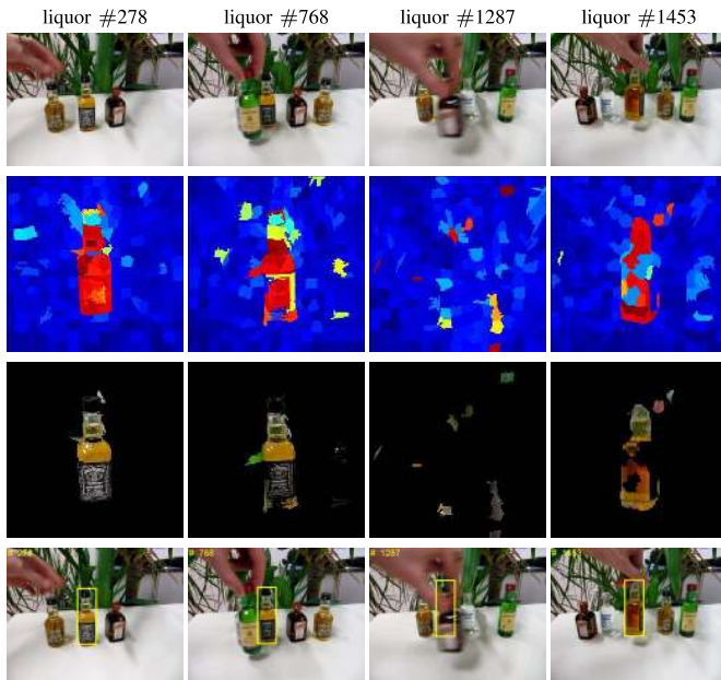
Fig. 10. Results of foreground/background segmentation and tracking across frames on sequence liquor . First row: original images. Second row: confidence maps of corresponding local regions, which is obtained by using the appearance model. Third row: the segmentation results. Fourth row: the final tracking results of each frame.
