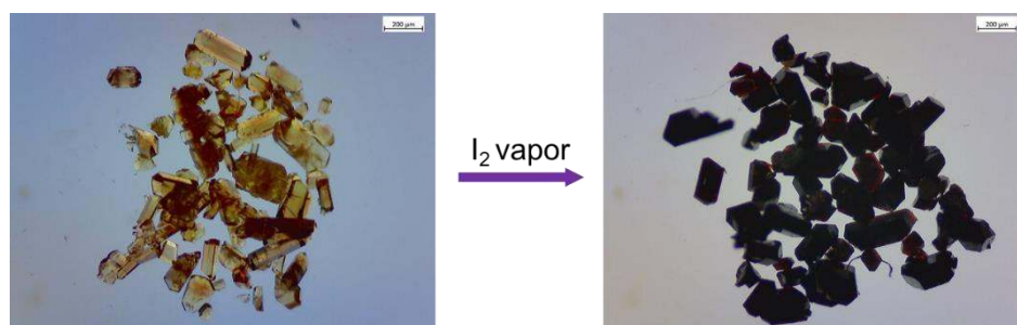
Supplementary Figure 14 Room light images of C3 before and after fuming with \text{I}_2 .
