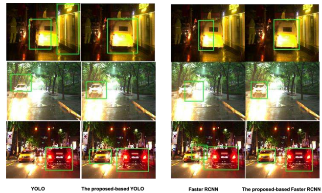
Fig. 8. Experimental results of the proposed system and Faster R-CNN [7] and YOLO [30] using the CCD Night dataset.
