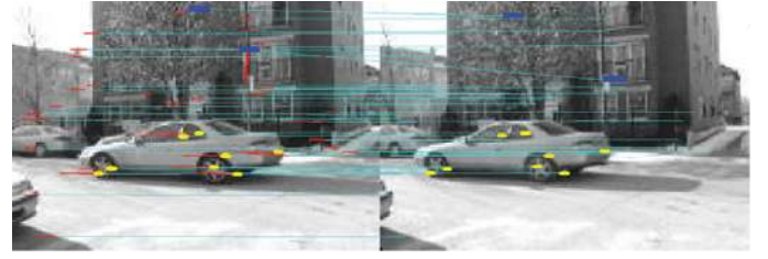
Fig. 1. SIFT correspondence from frame 200, 201 in outdoor sequence STREET . The lines across images represent the connections of features in two images, while the lines in the left frame represent the motion vector between them. The rectangles denote incorrect correspondences in the background. The circles denote correspondences from the moving objects.
