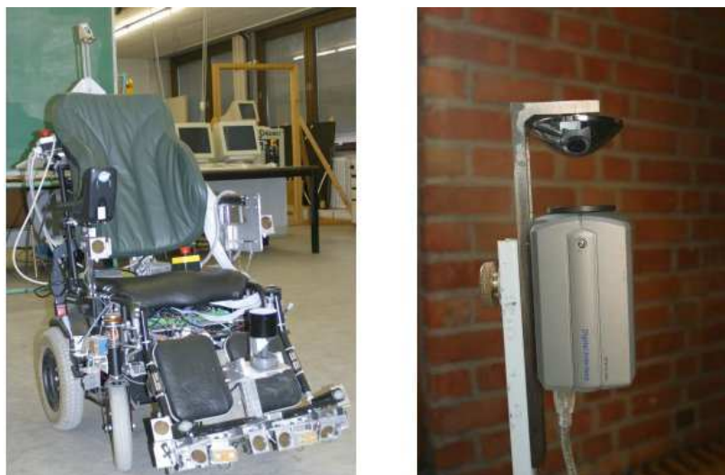
Figure 1. Left: the robotic wheelchair platform. Right: the omnidirectional camera, composed by a colour camera and an hyperbolic mirror
