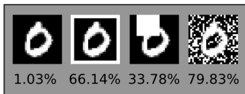
Figure 6.2: DBNs fail to be robust to various noise. The noise includes added borders, randomly placed occluding rectangles, and random pixels toggled to white.
