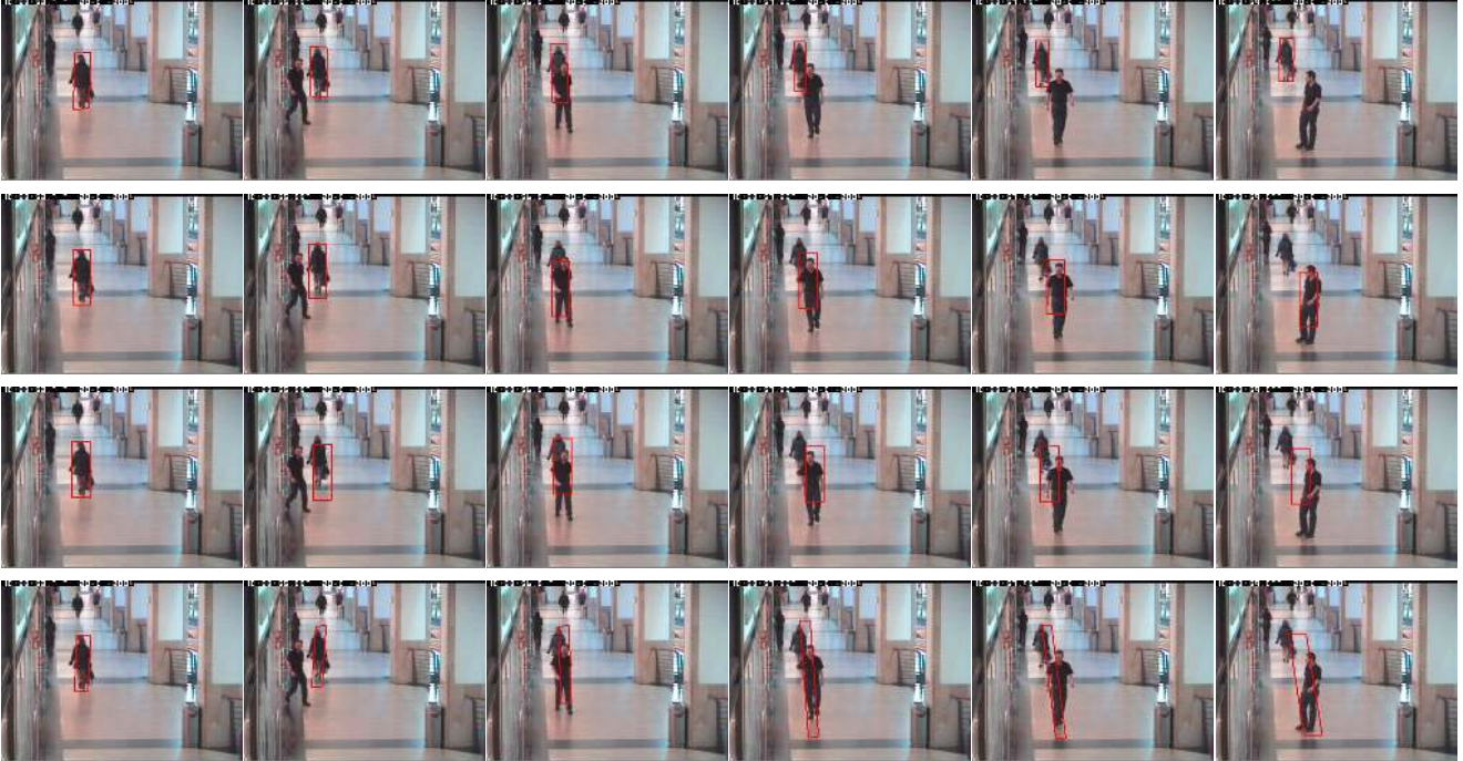
Figure 6. The tracking results of the third sequence: our proposed tracker (row 1), MS (row 2), CV (row 3), and AAPF (row 4) over representative frames with partial occlusion and background clutter.
