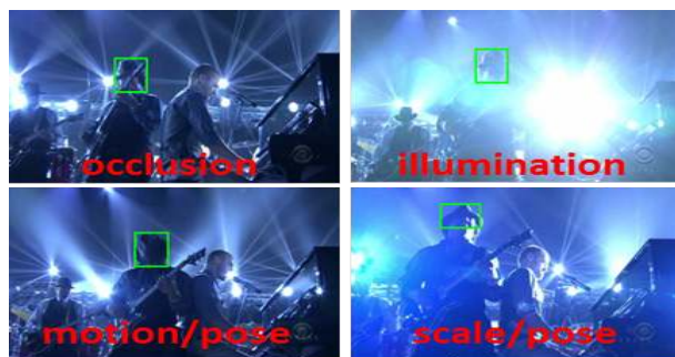
Figure 1. Frames from a shaking sequence. The ground truth track of the head is designated in green. Due to fast motion, occlusion, and changes in illumination, scale, and pose, visual object tracking is a difficult problem.
