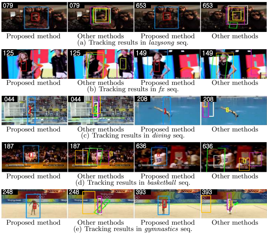
Fig. 7. Qualitative comparison of the tracking results with other state-of-the-art tracking methods. The red and blue boxes give the results of the proposed method (Combination of the IBB and OBB). The yellow, white, orange, green, and pink boxes give the results of MCMC method using the IBB representation, VTD, VTS, IVT, and MIL using the OBB representation, respectively.
