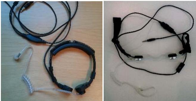
Fig. 1: Two of the throat microphones used in this study.
