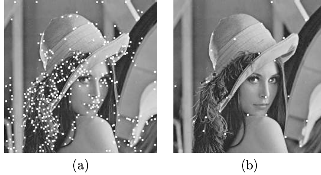
Figure 3. results of the detector (1): (a) without the local maximum criterion, with (b) the local maximum criterion.
