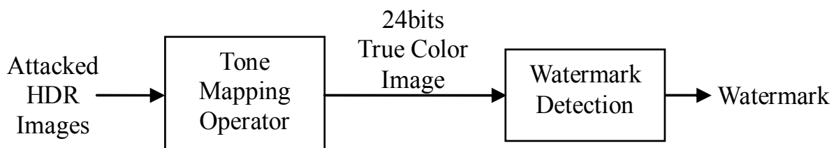
Fig. 2. The flowchart of the HDR image watermark retrieving procedure.
