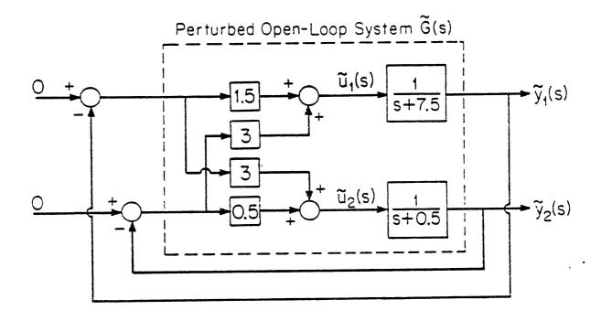
Figure 5: Perturbed feedback system (unstable).
